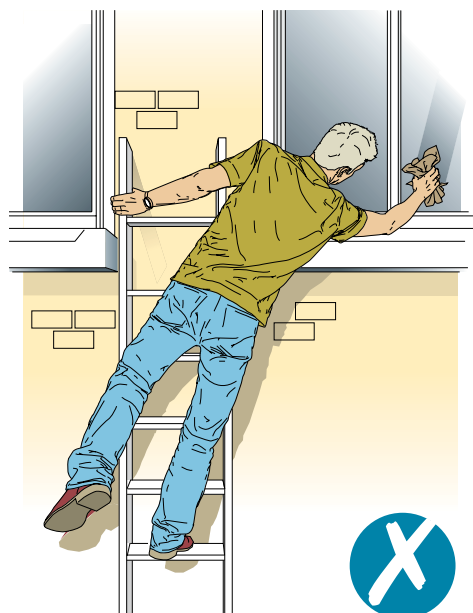
Figure 17a Incorrect - overreaching and not maintaining three points of contact
