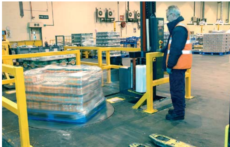
Figure 44 Stretch wrapping machine
