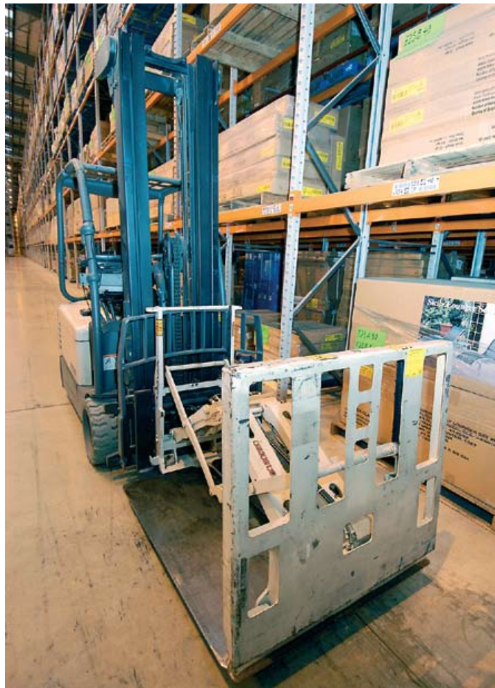
Figure 19 A fork-lift truck with push-pull attachment
