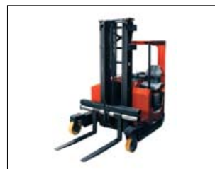
Figure 11 Bi- and multi-directional truck
