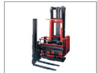
Figure 8 Very narrow aisle lateral and front stacking truck – man up
