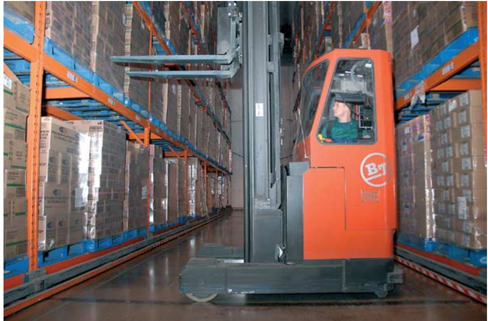
Figure 57 Reach truck with cold store customisation
