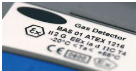
Figure 12 Ex marking showing that the equipment is explosion protected
