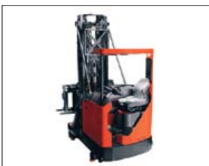
Figure 9 Very narrow aisle lateral and front stacking truck – man down
