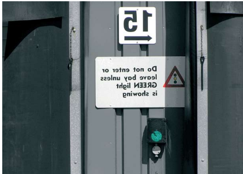
Figure 29(b) The writing on this additional sign has been reversed so it reads correctly when viewed by a driver in their rear-view mirror
